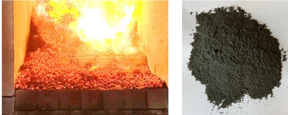
Figure 5: Pictures of ashes on the grate (left) and after de-ashing with a screw (right) during wheat straw combustion
