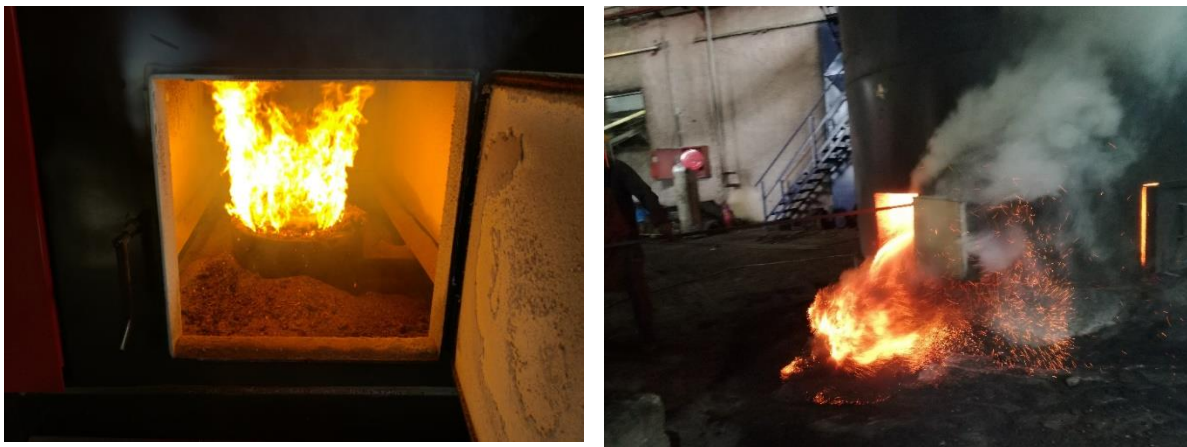
Figure 7: A fixed grate fed with underfed feeding (left), manual ash extraction from an operating fixed grate furnace [Image source: CETH].
