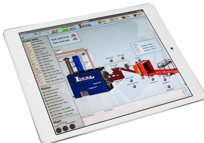
Figure 16: Example of a heating plant control and monitoring application (Image source: Linka 18 ).
