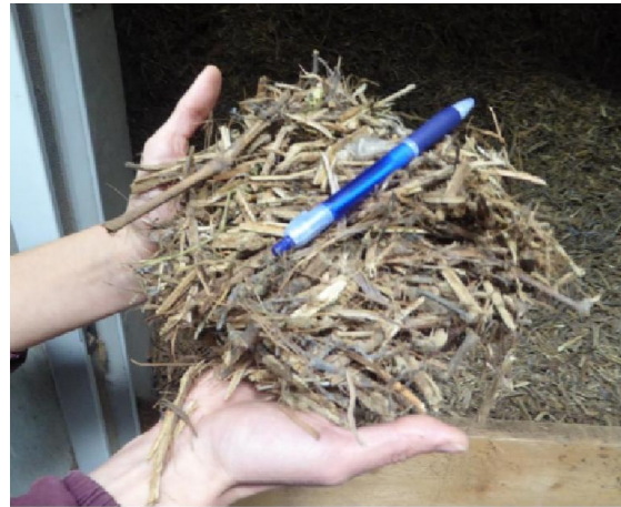
Vineyard pruning / hog fuel from integrated shredder / picker Particle size: G50
