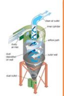
Dust control - Cyclones are conical containers that remove particulates from high speed rotating flue gas flows through vortex separation. Flue gas flows in a helical pattern before exiting the cyclone in a straight stream through the center of the cyclone and out the top. Particles in the rotating stream have too much inertia to follow and thus strike the outside wall, then fall to the bottom of the cyclone where they can be removed.
