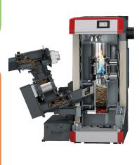
A revolutionary example of state of the art combustion systems with high fuel flexibility biomass are gasification boilers that include an updraft gasifier, a gas burner and a hot water boiler. Such systems can achieve almost zero CO and OGC emissions, significantly reduced NOx emissions (compared to conventional fixed-bed combustion technologies) and very low particulate matter emissions.
